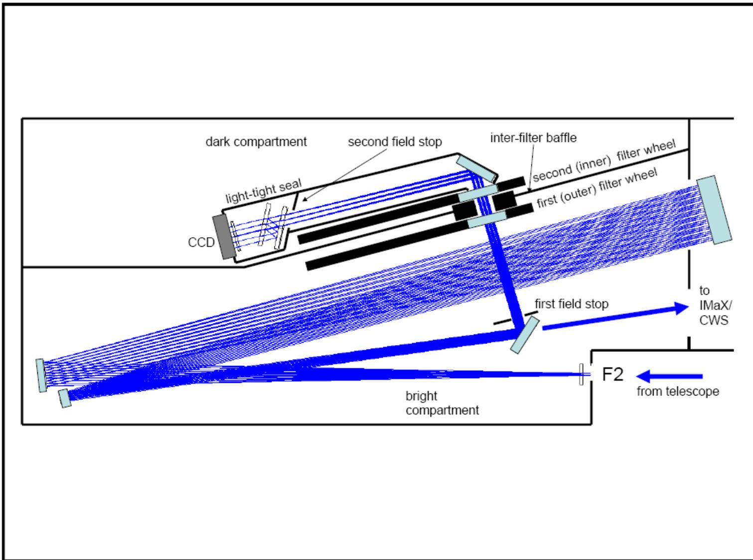
**Fig. 12.** Scheme of the baffling system of SUFI. The light tight innermost seal covers the light path after the second filtering, which is severely vulnerable to parasitic illumination. The double filter wheel separates the dark compartment from the bright compartment. Two consecutive field stops narrow the field which is propagated to the detector.
