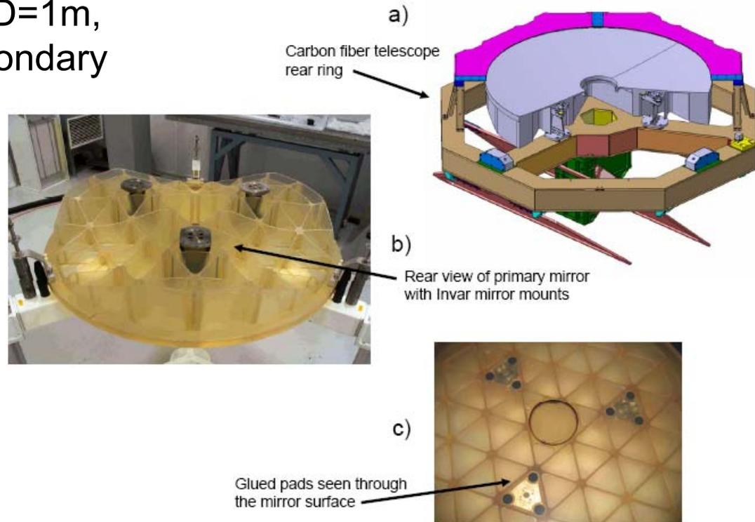
**Figure 4.** a) CAD model of the main mirror cell with the lightweighted ZERODUR mirror. The mirror is mounted with three flex blade fixation points to the carbon fiber structure, which forms the rear ring of the telescope. b) Backside view of main mirror after integration of the three flex blade fixation points. c) Glass/metal junction formed by glued Invar pads
