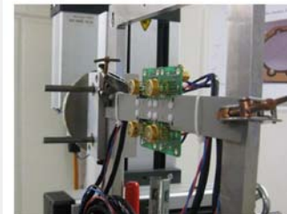
(c) PCB mounted on test frame, front view
