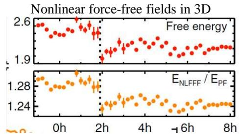
Monitoring of free magnetic energy before and after the X-class Flare (dotted vertical line) by a sequence of force-free equilibria. During the Flare magnetic energy is converted to thermal and kinetic energy => Dynamic phase, cannot be modelled by sequences of equilibria. Source: Sun et al., 2012
