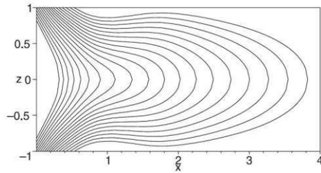
As in MHD,  $A(x,z)$  defines the magnetic field lines and the relation  $A \rightarrow J_y$  can be used to compute  $J_y(x,z)$ . (Picture from Schindler & Birn, JGR 2002)
