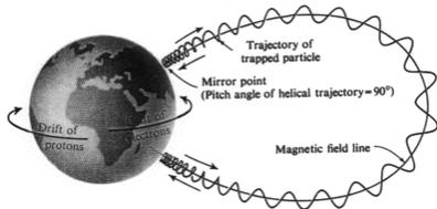
A *dipole magnetic field* has a field strength minimum at the equator and converging field lines at the polar regions (mirrors). Particles can be *trapped* in such a field. They perform *gyro*, *bounce* and *drift* motions.
