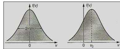
$$f(v) = n \left( \frac{m}{2\pi k_B T} \right)^{3/2} \exp \left( -\frac{m(v - v_0)^2}{2k_B T} \right)$$
