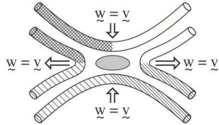
Breaking and rejoining of two flux tubes in 2-D to form two new flux tubes. Outside the diffusion region the flux-conserving velocity is identical with the plasma velocity.
