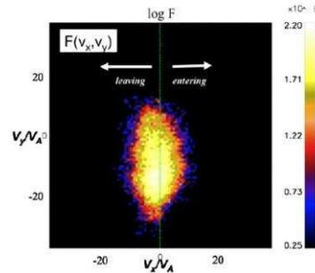
Reduced distribution  $F(v_x, v_y)$  in the outflow region. The distribution demonstrates the preferential loss of accelerated particles from the dissipation region. Source: Hesse et al. 2011
