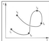
Many particles ( $i=1, N$ ) having time-dependent position  $x_i(t)$  and velocity  $v_i(t)$ . The particle path at subsequent times ( $t_1, \dots, t_3$ ) is a curve in phase space
