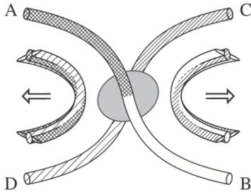
In 3D the flux-tubes not necessarily match perfectly. In 3D the flux-tubes break and rejoin only partly forming four new flux tubes.
