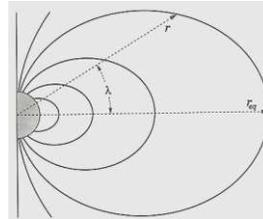
At distances not too far from the surface the Earth's magnetic field can be approximated by a *dipole field* with a moment:  $M_E = 8.05 \cdot 10^{22} \text{ Am}^2$
