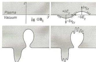
Consider a distortion of the boundary so the plasma density makes a sinusoidal excursion. The gravitational field causes an ion drift and current in the negative  $y$  direction,  $v_{iy} = -m_i g / (eB_0)$ , in which electrons do not participate; -> charge separation electric field  $\delta E_y$  evolves. Opposing drifts amplify the original distortions. The bubbles develop similar distortions on even smaller scales.
