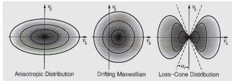
The most common anisotropic VDF in a uniform thermal plasma is the *bi-Maxwellian* distribution. Left figure shows a sketch of it, with  $T_{\perp} \neq T_{\parallel}$
