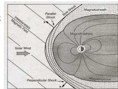
The most famous and mostly researched shock is the **bow shock** standing in front of the Earth as result of the interaction of the **magnetosphere** with the **supersonic solar wind**, with a high Machnumber,  $M_s \gg 1$ . Solar wind density and field jump by about a factor of 4 into the **magnetosheath**.
