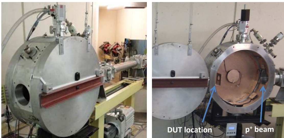
Figure 6.13. Displacement damage radiation campaign: setup. A beam line communicates the cyclotron, where the protons are generated, with a small vacuum chamber where the DUT is located (left picture shows beam line and chamber). Right photo displays the open chamber. Protons enter the chamber through the right aperture and hit the device located on the left side.
