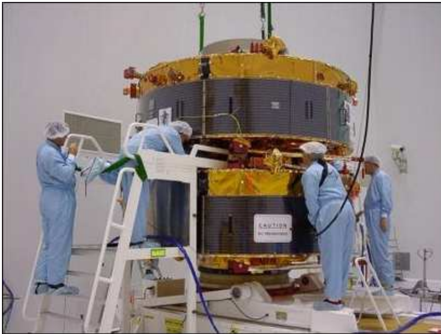
Figure 3.2: Cluster 1 (top) and Cluster 4 (bottom) in a clean room (Courtesy of ESA).
