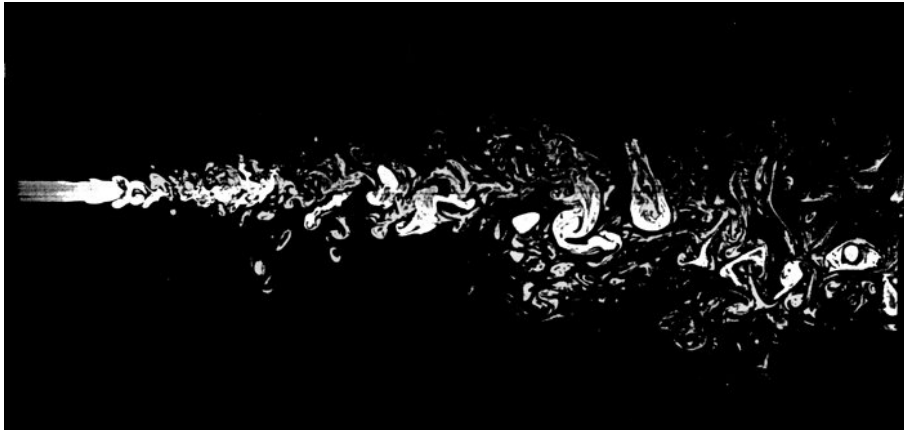
Figure 2.6: Turbulent water jet ( Van Dyke 1982). Photograph P. Dimotakis, R. Lye and D. Papantoniou.
