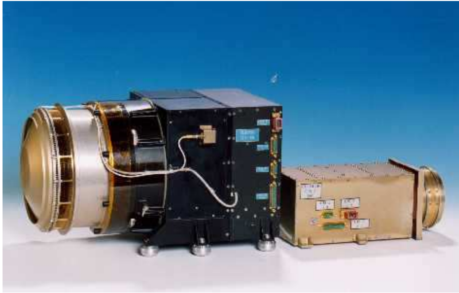
Figure 3.5: CODIF (on the left) and HIA (on the right) ion detectors of the CIS experiment (Courtesy of H. Rème).
