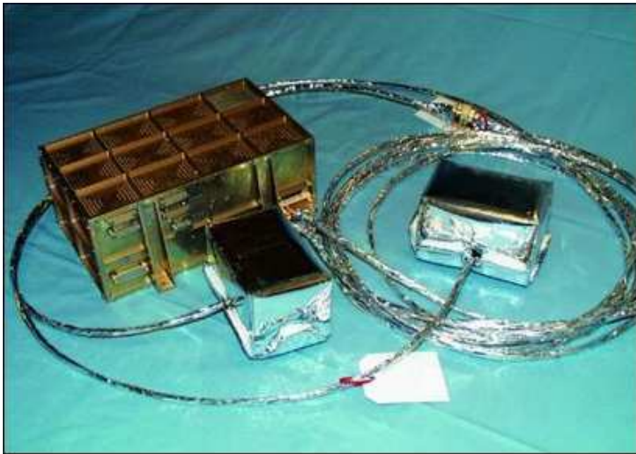
Figure 3.4: Fluxgate Magnetometer for the Cluster spacecraft consisting of Digital Processing Unit (DPU, left), outbound sensor with a long cable (right) and inbound sensor (middle, Courtesy of A. Balogh and E. Lucek).
